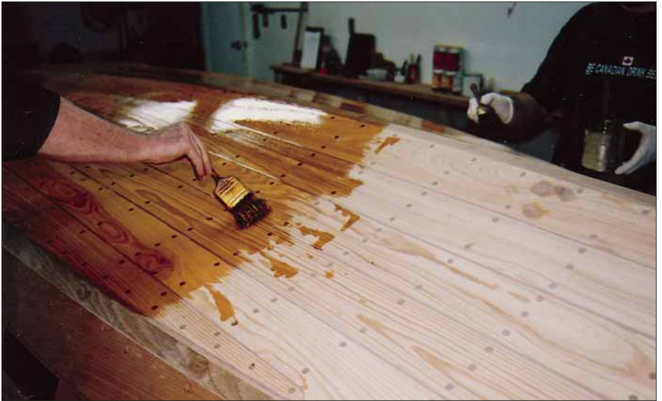
The first coat of varnish changes the colour dramatically. The boat will have many more coats before it is complete.
