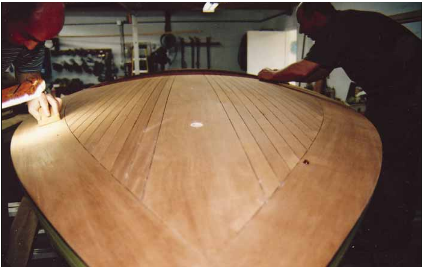
Before a coat of varnish can be applied, the builders at Brackley Boats undertake a final sanding. The lights help show any imperfections that still need to be addressed.
