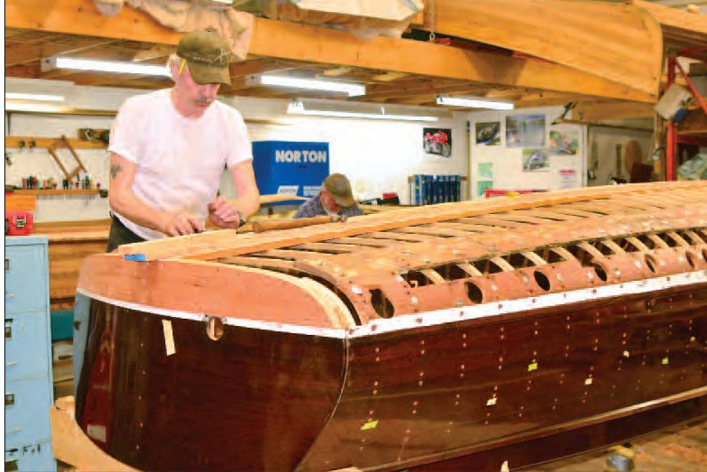
Rob Gerigs works on *Little One* (above). The boat needed a new bottom after 90 years of use. *Little One*, a 1919 Minett, is powered by a very rare Buchanan Bull Dog engine (below).
