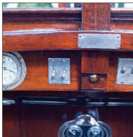
The dash has a Minett plaque, simple gauges and a removable wind up clock.
